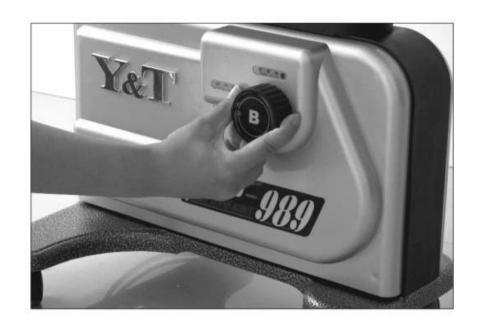
When choosing to make the ball shoot randomly, first turn knob A to move its red dot to the alternative course position (see page 8). Then turn knob B to move its red dot to the random point position. The robot will shoot the ball out randomly in this way. If turning the knob B to move its red dot to standard point position, the ball shooting position will back to regular alternative point position.
